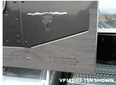
VP142103 PB SLEEPER EXTENSION PANEL - 1987 & NEWER - 379, 388, 389 - 70"/78" - BLANK
