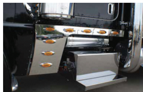
VP150104 PB - 379, 388, 389 BATTERY BOX - ALUMINUM
